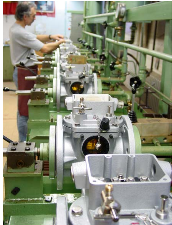
Figure 8: Functional and leakage test
