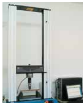
Universal Testing Machine Max. Capacity: 50 kN
