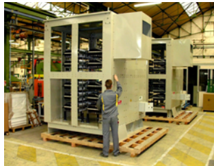
Neutral Earthing resistor, Saudi Arabia.
