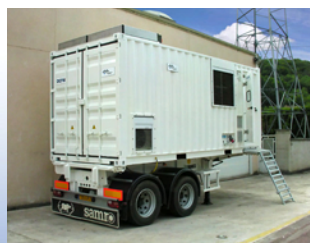
Mobile load bank of 1875 kVA on road trailer.
