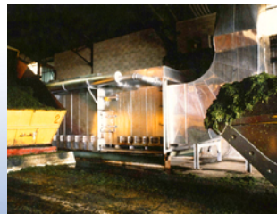
Air heating resistors for dehydrating alfalfa.
